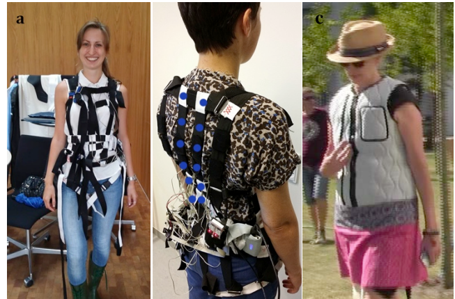
Figure 2. The vibrotactile vest: adjustable harness (a) front and (b) back and (c) outer shell and skirt-apron.
