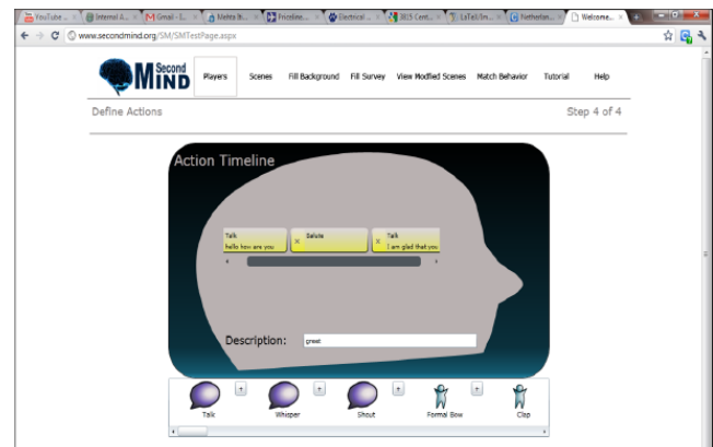
Figure 1. Authoring a greeting behavior as a left-to-right sequence of basic actions “talk (text)”, “salute” and “talk (text)” on the timeline.
