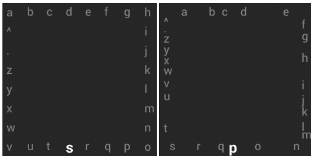
Figure 4: Normal target size for letters (left) and adjusted target sizes (right) depending on letter frequencies.
