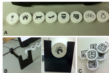
Figure 3: (a) Tangible pieces used in the experiment; (b) The webcam device used to recognize the fiducials; (c) Fiducials engraved at the back of the pieces
